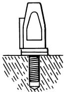
**c.** On metal or fiberglass masts, drill hole 1/4" (6.5 mm) and tap 5/16" (8 mm) x 18. Fit securely using washers as shown above, and use glue (epoxy or thread lock) on threads for permanent mounting.
